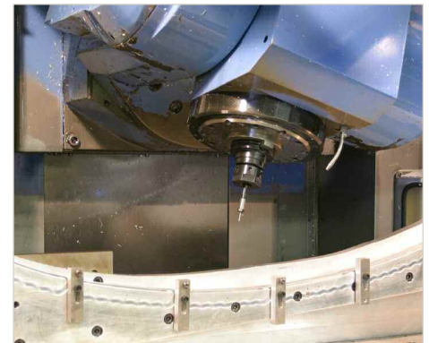
Closeup view of a titanium structural part being machined on a Mazak Vortex 815 at Hansen Engineering.
