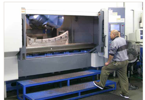
Mazak Vortex 815 is set up to run a part at Hansen Engineering. The machine is a dual pallet system with a 5-axis, 50-hp, 10,000 rpm spindle. It is equipped with a 60-tool magazine and is operated by a Fanuc 15i controller. Work envelope is 120"x31.89"x24" XYZ.
