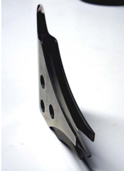
Matrix Systems supplies complex parts in short runs, such as this roller guide for a custom packaging machine.
