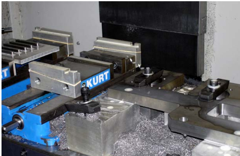
Efficient setups and quick turnaround are essential to Nguyen's success. Here three jobs are set up in the Nexus VCN-510C.
