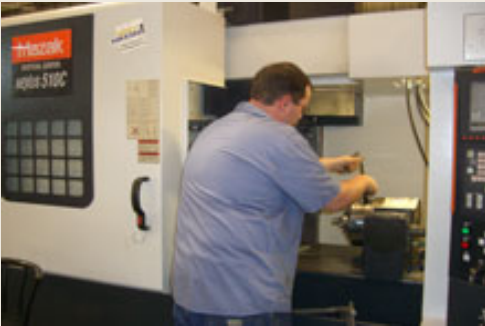
An index table on the Vertical Center Nexus 510-C allows part setup while the machine is running.
